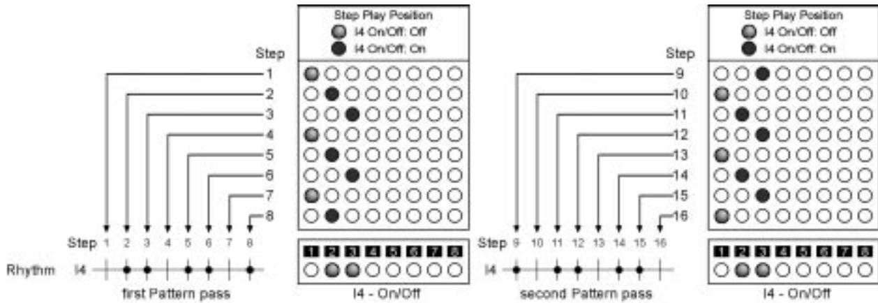
Result: During the two passes of the Pattern different rhythms are generated although the actual Pattern rhythm (On/Off track for I4) remains the same. At the end of the third pass (after 24 Steps) the Step Play Position has again reached Step 1 and the same rhythm as in pass 1 is generated; the whole cycle starts over here.
