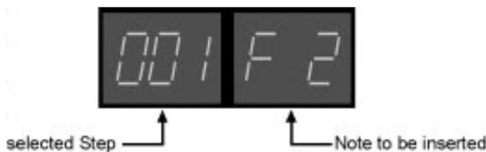
Use the up/down buttons (step buttons 11 and 12) to enter the value for the note you want to insert. Press Enter to insert the notes into all selected steps press "Exit" to return to step selection.
