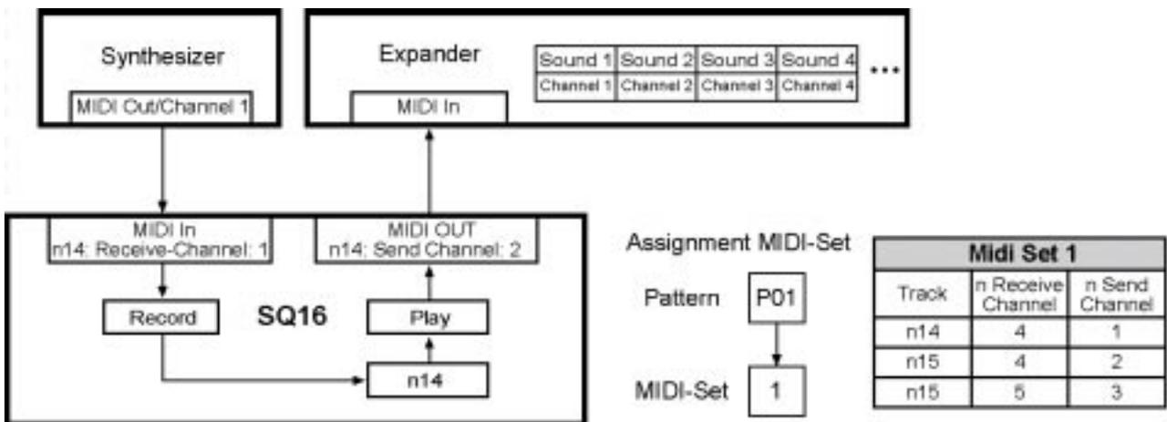
As an example, you want to record onto note track 14 in pattern 1 from a keyboard which is sending on channel 1; for playback you want to use sound 3 in the expander. MIDI Set 1 contains the necessary settings for this; you then need to assign MIDI Set 1 to Pattern 1.
