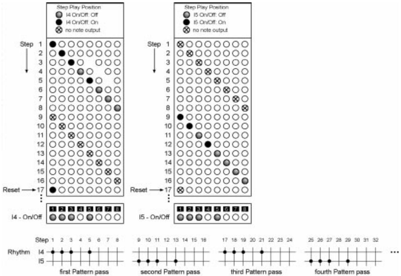
During the first pattern pass (step 1 to 8) instrument I4 is played normally while the output for instrument I5 is suppressed. During the second pass I4's output is suppressed while I5 plays normally. This switches for any subsequent pattern pass.
