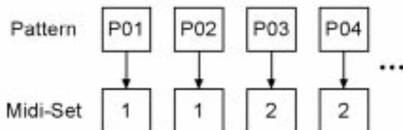
Depending on the settings made in the MIDI Set the Patterns use different note numbers and MIDI channels (instrument tracks) or different MIDI send channels and MIDI receive channels (note tracks). Patterns 1 and 2 play back instrument tracks 1...4 on MIDI channel 10; Patterns 3 and 4 play back instrument tracks 1...4 on MIDI channel 16. Additionally, Patterns 1 and 2 use different note numbers for instrument tracks 1...4 than Patterns 3 and 4.
