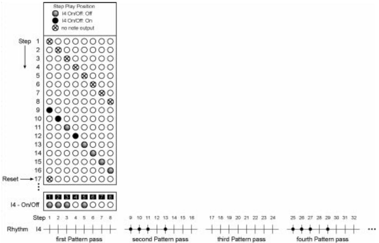
For the first 8 steps the output is suppressed; for the next 8 steps the notes play normally. After 16 steps (Reset) at step 17 the output is again suppressed and everything starts over.
