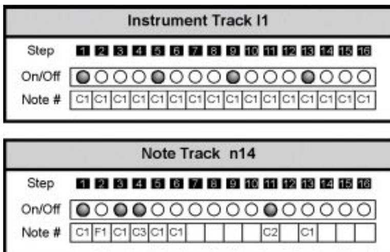
The instrument track I1 outputs notes only on steps 1, 5, 9 and 13; the note track n14 only on steps 1, 3, 4 and 11.
