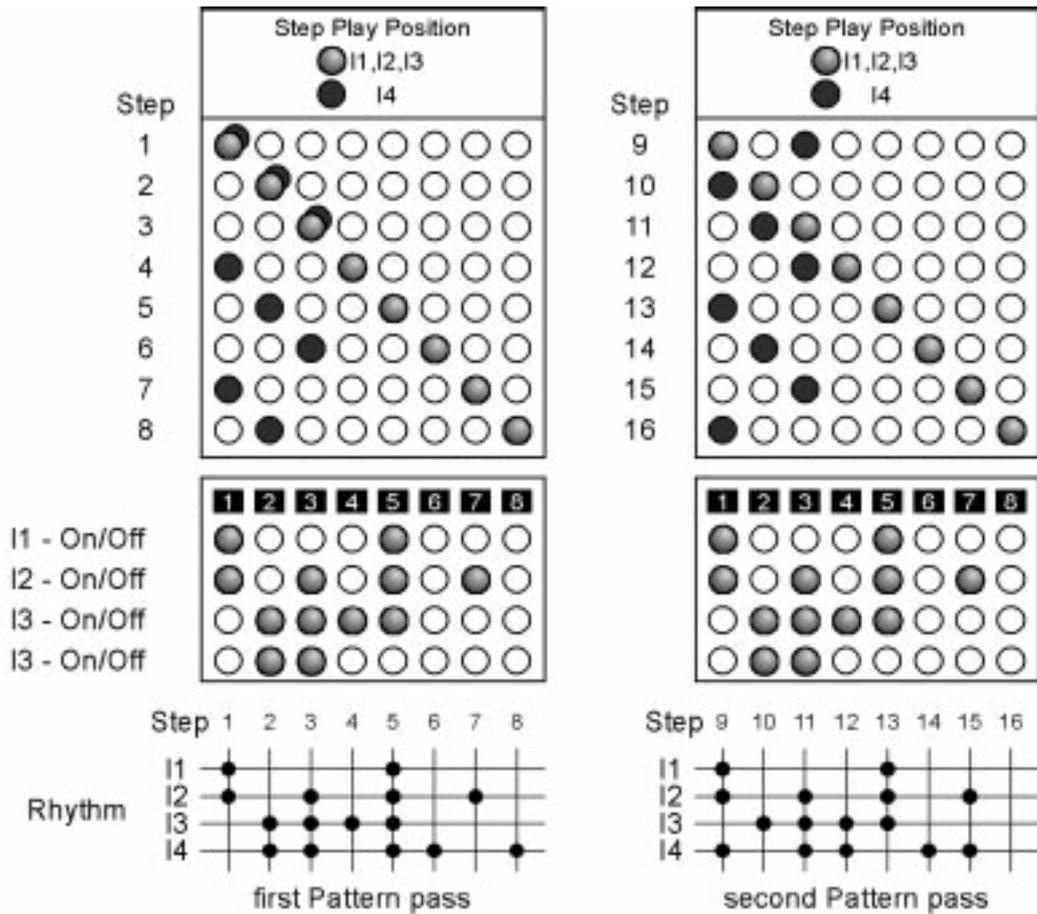
For Instruments I1...I3 each pass results in the same rhythm and the same Pattern Play Position while Instrument I4 uses different Pattern Play Positions and hereby generates a different rhythm.
