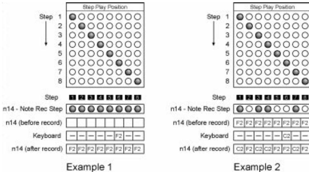
In example 1 the note F2 is recorded into all steps. For example 2 the step recording tracks was changed so that only Steps 1, 2, 3 and 7 are recorded; Steps 2, 5, 6 and 8 remain unchanged.
