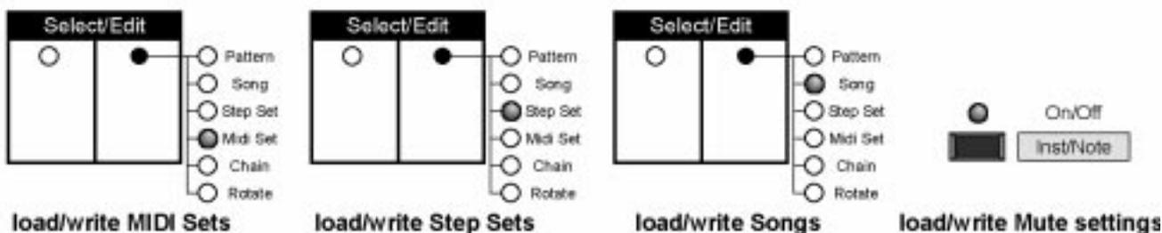
3. Select the Block you want to load from or you want to write into with the up/down buttons (step buttons 11 and 12); the left display shows the appropriate Block 1...8.
