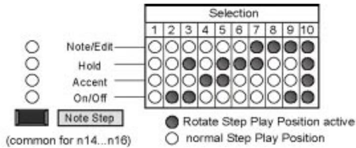
The LED's indicate which data is affected by the Rotate setting. The Destination value is common for all note tracks.
