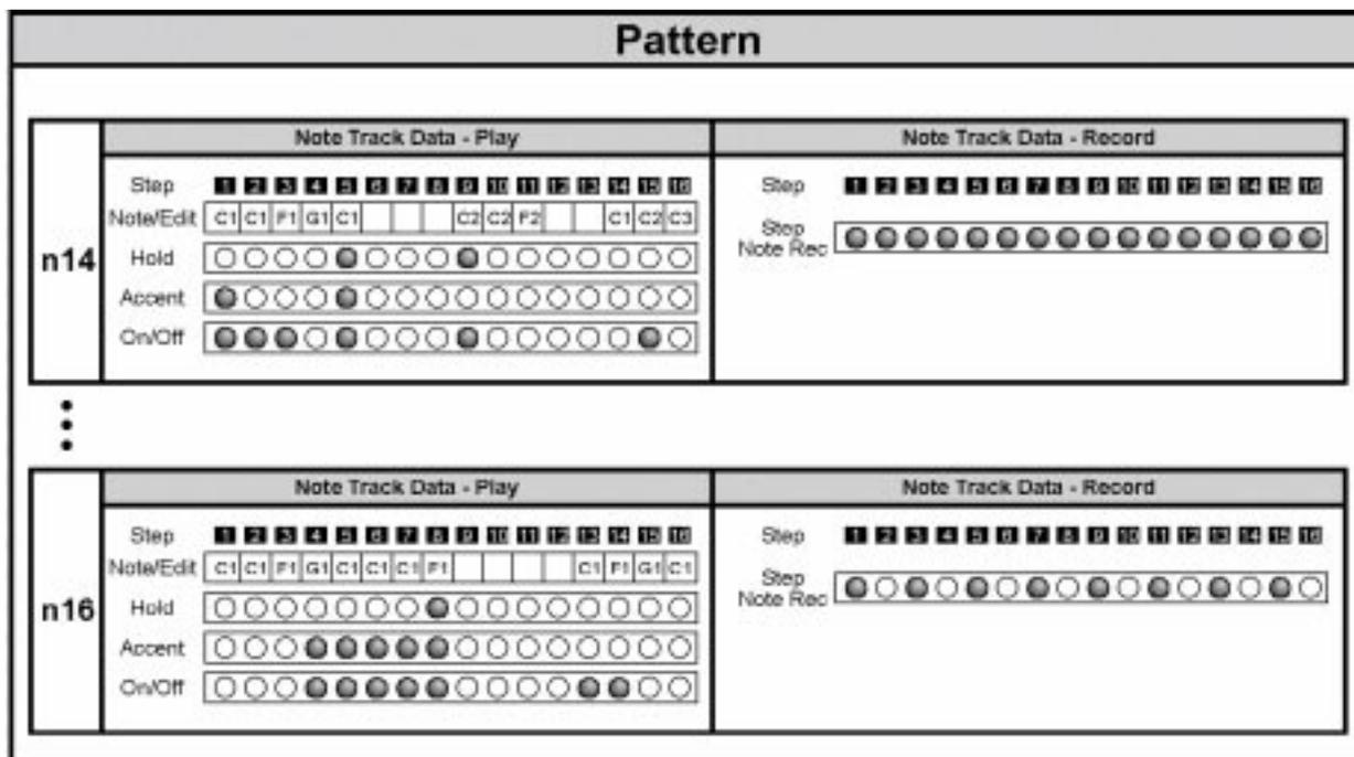
A note track contains data related to the playback or recording of this track. The track "Note - Rec Step" determines into which steps of the note track notes can be recorded (see 11.1.3). Here's a description of the playback data:
