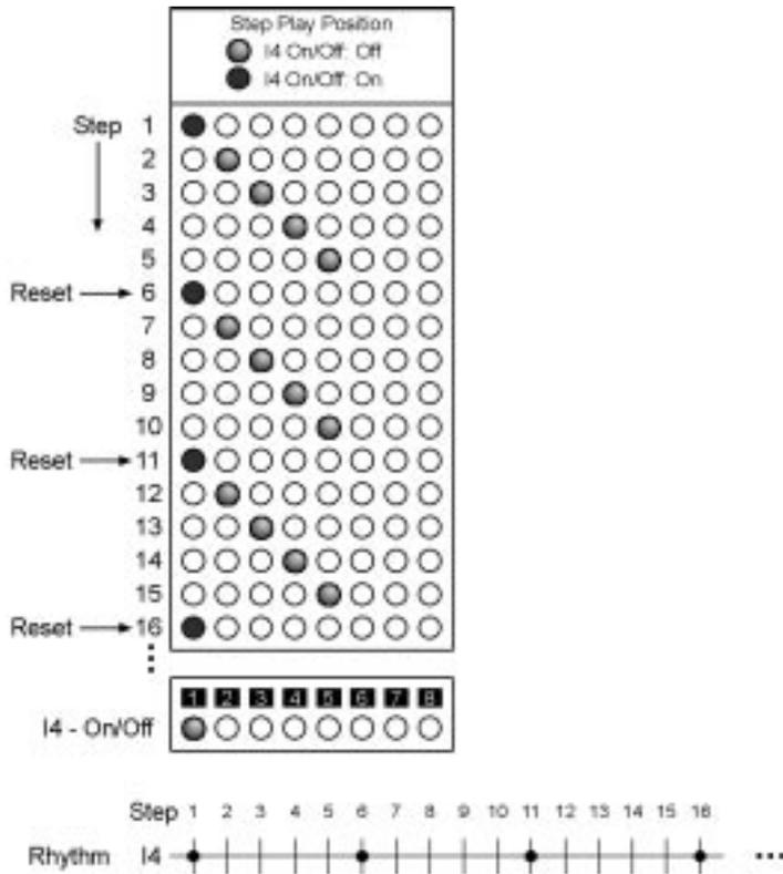
If Shift = 0 the Step Play Position is incremented for each Step as usual by one; the Delay setting isn't used here. Every 5 steps a Reset to Step 1 takes place; this makes Instrument I4 react as if its Pattern Length would be 5 steps. All other instruments without Rotate use the normal Pattern Length of 8 steps. You can use this mode to create different meters for various tracks.
