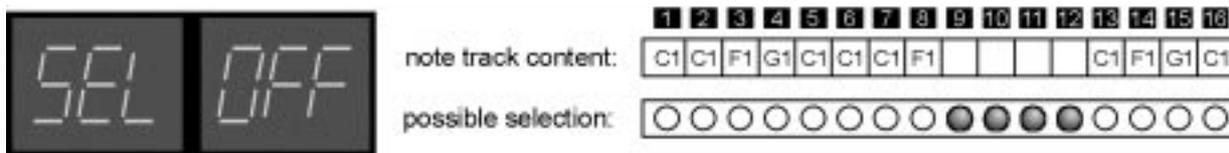
All steps containing no notes blink short. You can use the step buttons to select one or more of those steps. The selected steps light permanently. In the above example the "ALL ON" button was used to select all empty steps.
