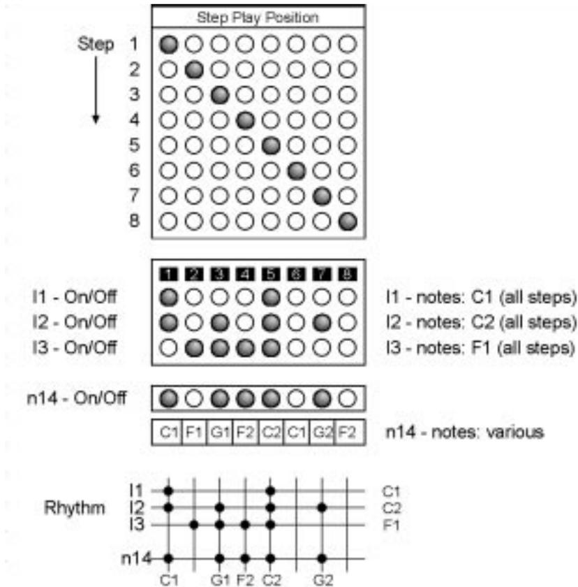
When playing back a pattern all steps are played sequentially starting with step 1. Each pattern has its own pattern Length, e.g. a number of steps after which the pattern starts over. In the above example the pattern length is 8 steps; the pattern is playing Step 1, 2, 3...8 and then starts from the beginning. The Step Play Position is the currently playing step within the pattern.
