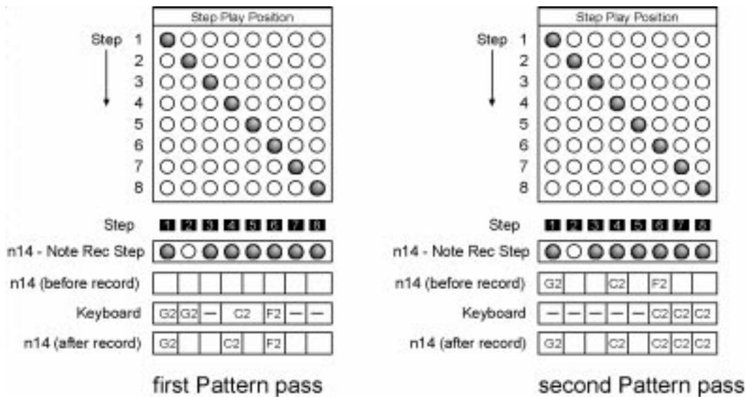
During the first pass Steps 1, 4 and 6 are recorded. Step 2 isn't recorded because it isn't set to "On" in the Step recording track. Note C2 is held over Steps 4 and 5 and only recorded in Step 4. During the second pass Step 6 is overwritten and Steps 7 and 8 are newly recorded.
