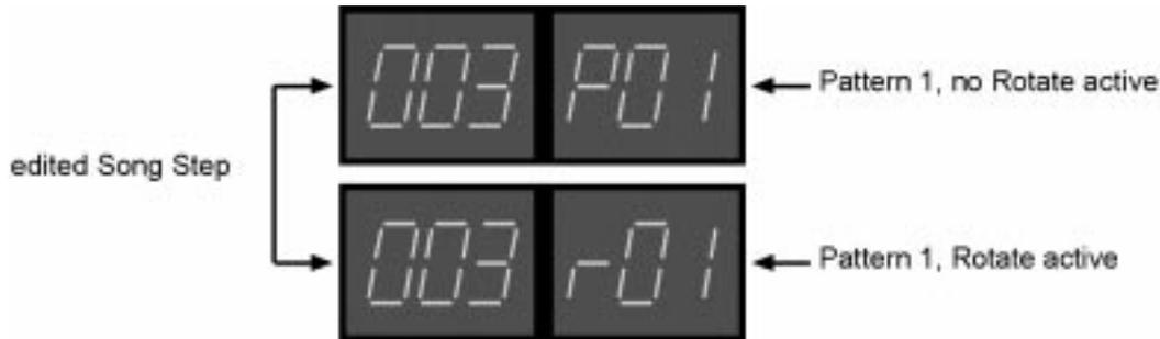
**Please note:** The function Song Edit - Rotate is used to select which Rotate setting is active.
