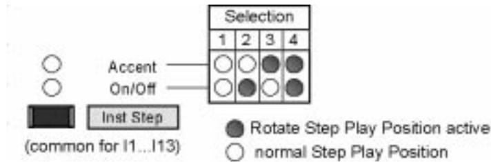
The LED's indicate which data is affected by the Rotate setting. The Destination value is common for all instrument tracks.
