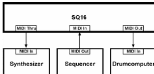
Here the SQ16 gets synchronized from an external sequencer. The SQ16 in turn controls the computer. If the external sequencer must control the synthesizer too, this can be done via the MIDI Thru of the SQ16 in case the external sequencer has just a single output.
