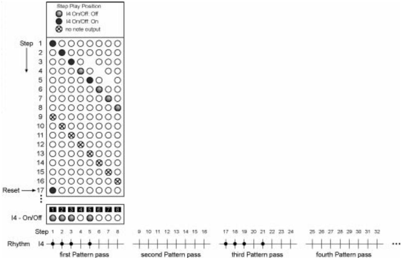
For the first 8 steps (Delay) the notes play normally, for the next 8 steps the output is suppressed. After 16 steps (Reset) with Step 17 the notes start again playing and everything starts over. By using different values for Reset and Delay you can generate different rhythmical structures, like:
