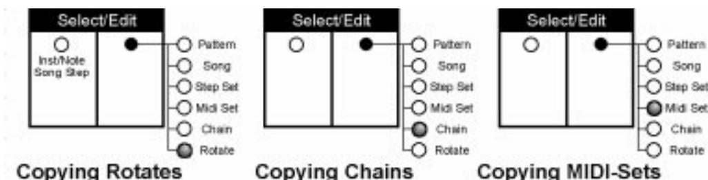
2. Select which Rotate/Chain/MIDI Set/Step Set or Song shall be copied: Keep pressed the "Select" button in the right Select/Edit section and press step button 1...16 for the desired selection (step button 1...8 when copying Songs).
