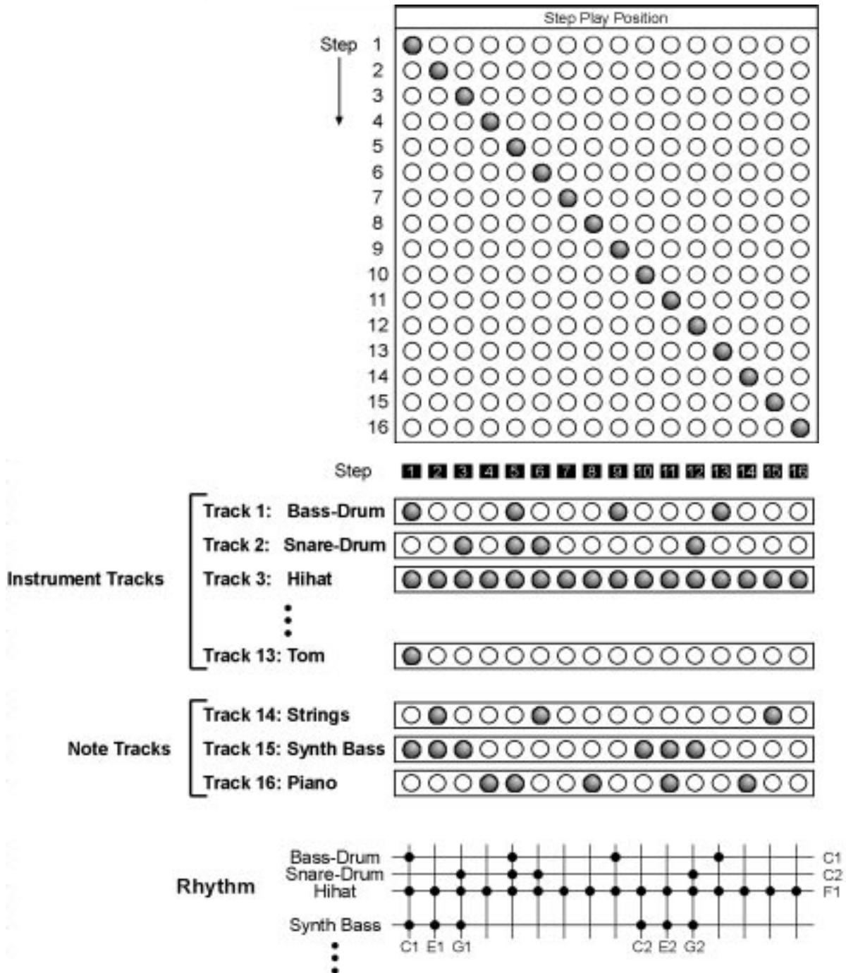
Each pattern contains 16 tracks. Each track contains exactly one note per step. Within each instrument track all notes are the same. If the SQ16 is triggering a drum expander each instrument track plays a single drum instrument (drum expanders usually are built around drumsets in which each note is assigned to exactly one instrument).
