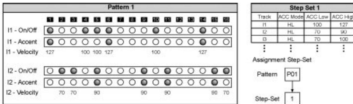
Each Step Set contains an ACC Mode setting for each instrument track. The setting "HL" means that all steps use either the ACC-Low value (accent not active) or the ACC-High value (accent active). There exist other ACC modes that are used to trigger echoes (delays). A detailed description of the ACC modes can be found in section 6.3.1. This section also describes the various possibilities of the Step Sets.
