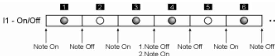
All sent Note On/Off commands have the same note number and the same MIDI channel. At the beginning of the current play step (On/Off = On) is always sent a Note On command; at the end of the Step a Note Off command. If several subsequent steps are active first a Note Off command is sent and immediately after it a Note On Command (see Step 3 -> Step 4 in the above example).
