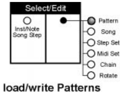
3. Select the Block you want to load from or you want to write into with the up/down buttons (step buttons 11 and 12); the left display shows the appropriate Block 1...8.
