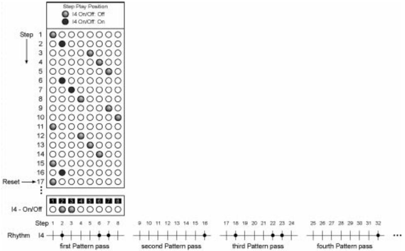
Up to including step 16 the rhythm is similar to the one in example 1 for mode d. After 16 steps (at step 17) a Reset is performed and the whole Rotate starts over. The next Reset again takes place after 16 steps (at Step 33). The rhythm repeats itself every 2 Pattern passes and so is running in sync to the normal Pattern rhythms (without Rotate).
