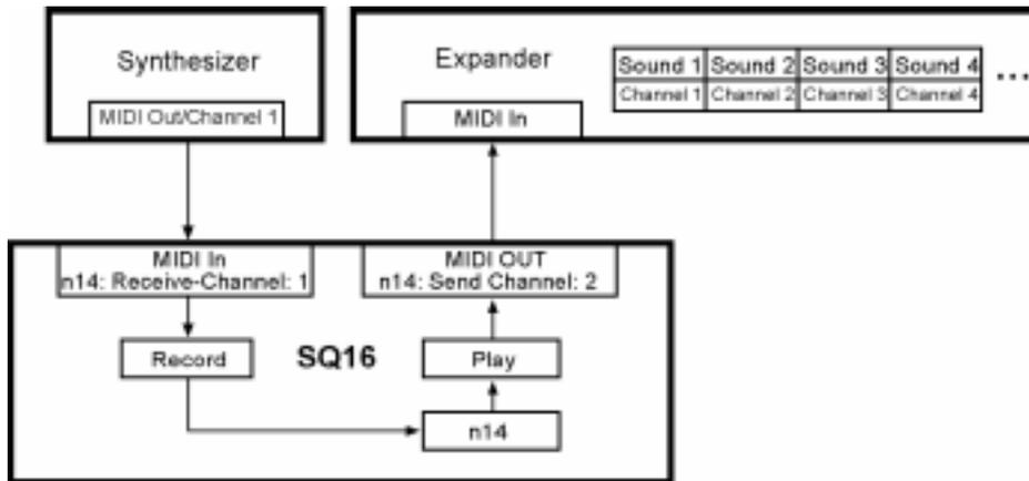
For example, you want to use an external synthesizer to record note data on note track 14 (for recording note tracks see section 11). Since the synthesizer is sending on MIDI channel 1 the MIDI receive channel for note track 14 must also be set to 1. When playing back note track 14 you want it to use the sound on MIDI channel 2 in the connected expander; that's why you must set the MIDI send channel to 2.
