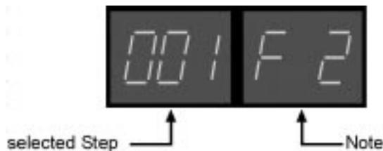
Use the up/down buttons (step buttons 11 and 12) to edit the note of the selected step. All edits take place immediately and must not be confirmed with "Enter". Press "Exit" to return to step selection.
