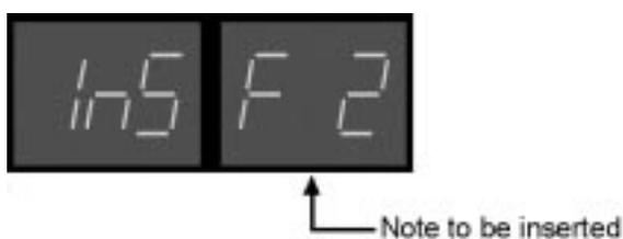
The right display shows the note number you are about to insert. Use the up/down buttons (step buttons 11 and 12) to enter the desired value. Press the Enter button to insert the notes or Exit to return to step selection.
