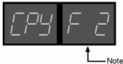
Use the up/down buttons (step buttons 11 and 12) to enter the desired common note number. Press the Enter button to set all selected notes to the same note number or the Exit button to return to the step selection.
