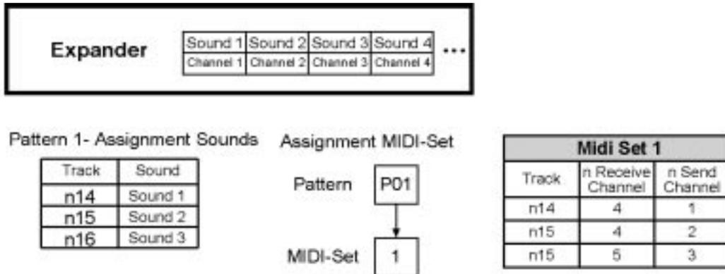
The note tracks n14, n15 and n16 from Pattern 1 shall play different sounds from a connected expander. Pattern 1 is assigned a certain MIDI Set, for example MIDI Set 1. To achieve the desired sound assignment for Pattern 1 you need to make the appropriate settings in MIDI Set 1 for the MIDI send channels (n send channel).
