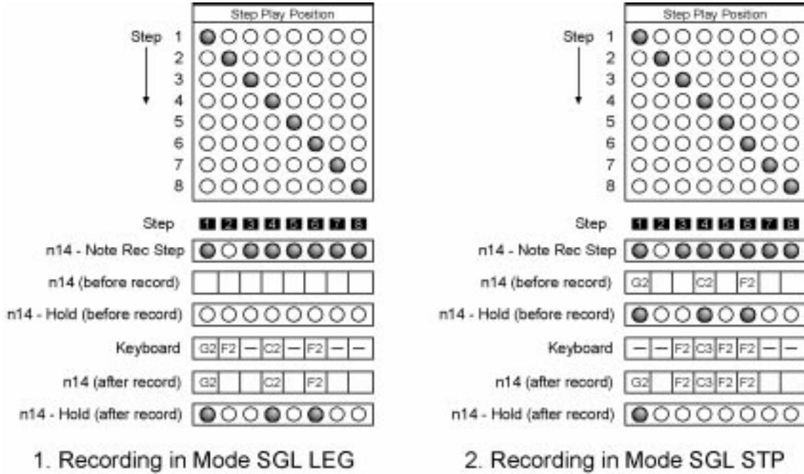
During the first pass Steps 1, 4 and 6 are recorded and simultaneously Hold is also set for Steps 1, 4 and 6. After this the recording continues in mode SGL STP; Steps 3...6 are recorded now and Hold is again turned off for Steps 4 and 6. Since Step 1 isn't recorded again Hold stays active for this Step.
