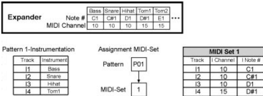
The instrument tracks I1...I4 from Pattern 1 shall play certain instruments in the connected expander (Pattern 1 - instrumentation). Pattern 1 is assigned a certain MIDI Set, for example MIDI Set 1. To achieve the desired instrumentation for Pattern 1 you have to make the necessary settings in MIDI Set 1 to match the instrument tracks and the desired MIDI channels and note numbers.
