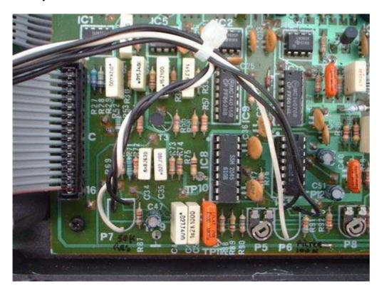
Remove trimmer pots P6, 7 and 3. Solder wires to the empy solder points and connect the other side to the external potmeters.
