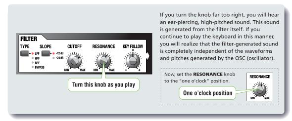
on a piano, its initial sound would include most of the harmonics that generates bright sound. Afterward, the sound would fade gradually, as a decrease in harmonics will result in a dull (dark) sound. To re-create this phenomenon, create a time-varied effect with the filter. In other words, the operation of turning the [CUTOFF] knob becomes automated as you play the keyboard.
