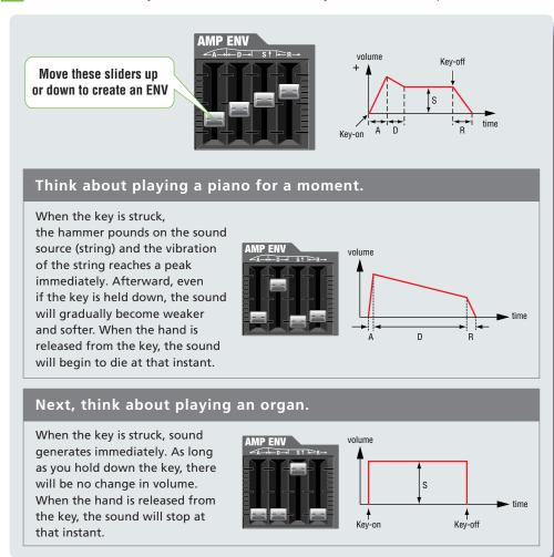
Move these [A], [D], [S], and [R] sliders up and down, and listen to how it affects the sound. Afterward, to leave some lingering sound after releasing the hand, leave the [R] slider at the mid-high position.
