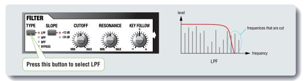
I urn the **[CUTOFF]** knob as you play. Slowly turn it counter clockwise from all the way right (MAX) leftward to (MIN). The sound will gradually muffle during this process, and when it is turned left all the way, most of the sound becomes inaudible. This is due to the fact that most of the sound frequencies have been filtered out and rejected.
