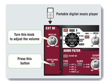
Next, press the [FILTER ON] button. Press the [TYPE] button, and select LPF(\*1). The LPF filters out the user-defined range of high frequencies that pass through. This has no effect on the low frequencies.
