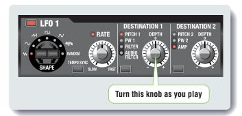
You can switch the vibrato waveform by pressing the **[SHAPE]** button. Additionally, turning the **[RATE]** knob will change the speed of vibrato. Try out various settings for vibrato with different waveforms and speeds. For example, the human voice or a violin would typically have a vibrato rate of 2 to 7 cycles per second.
