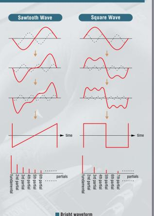
Brighter sounds include many high frequency harmonics; darker (rounder) include more of the low frequency harmonics. There is a technique called subtractive synthesis method in which harmonic elements are cut to change the brightness (waveform) of the sound. It is a popular method for creating composite waveforms. The SH-201 has waveforms with built-in harmonics. These waveforms with harmonics components are rejected through the filter to change the brightness of the sound.
