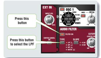
I urn the [CUTOFF] and [RESONANCE] knobs gradually left or right, and hear how the sound changes. Afterward, turn the [CUTOFF] knob all the way left to (MIN). The sound now will be inaudible, as most of the frequency range is blocked.
