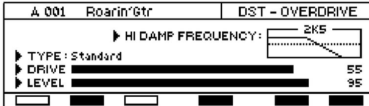
Type parameter. Range: Standard, UK Tubes, US Tubes, Modern ovd, Hot Tubes, Flattened, Brite Tube, MOS-FET#1, MOS-FET#2, MOS-FET#3.
