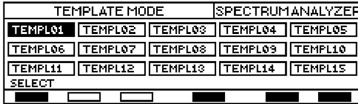
After selecting the Template with the VALUE knob, press WRITE to save the results of the analysis or SELECT (Edit) to compare the current analysis with that in the memory selected (by default, all the Template memories are empty)
