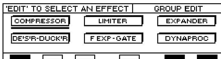
When the compressor group is selected and editing of the COMPRESSOR effect is activated, the following video page will appear on the display:
