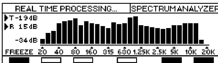
The press FREEZE (Edit) to block the analysis. By rotating the VALUE knob it will also be possible to obtain a numerical reading of the results of the analysis for each of the 31 bands.
