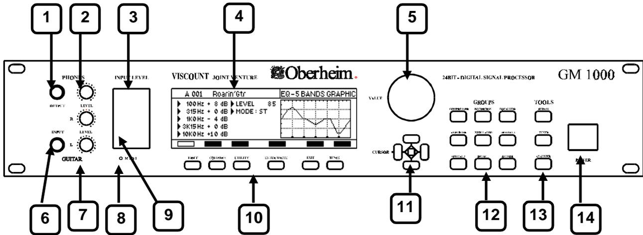
1. **Phones Output:** this socket is a headphones output which allows the GM 1000 to be used even without connection to an amplification system.
