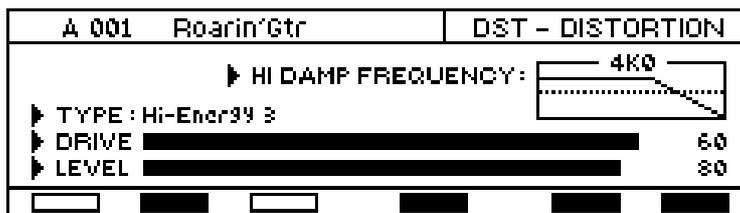
Type parameter. Range: Standard 1, Standard 2, Standard 3, Mellow 1, Mellow 2, Mellow 3, Boosted 1, Boosted 2, Heavy Tube 1, Heavy Tube 2, Heavy Tube 3, Hi-Energy 1, Hi-Energy 2, Hi-Energy 3, Hi-Energy 4.
