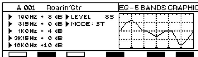
100 Hz, 315 Hz, 1K Hz, 3K15 Hz, 10k parameters. Range: -14 +14 dB.
