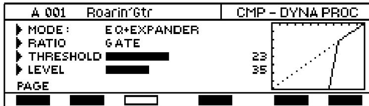
Mode parameter. Range: Dynamic Loudness, Spectral Compressor, Spectral DeEsser, Spectral Exp/Gate, Eq + Compressor, Eq + Expander.
