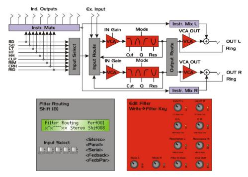
The filter always works in parallel to the rest of the audio engine and is always present at the stereo mix (see picture).
