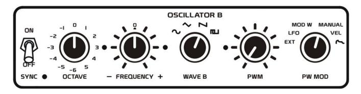
PULSE WIDTH MODULATION AMOUNT: The PWM control sets the amount of modulation that the PW MOD source will have on Oscillator B's square/pulse waveform. When this control is rotated fully counter-clockwise, no modulation of the square/pulse wave will occur producing a true square wave. As you rotate this control clockwise, the affect of modulation will increase, causing the square wave to narrow its pulse width duration.
