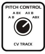
In the **A B** position, both oscillators will be controlled by MIDI notes received. In the **A BX** position, Oscillator A will respond to MIDI notes received, while Oscillator B will be controlled by an external voltage inserted into the CV IN jack.
