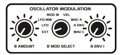
The A ENV setting lets Envelope 1 control the amplitude of Oscillator A's waveform, as determined by the WAVE A control setting, to modulate Oscillator B's frequency. This provides a more traditional form of FM where the modulation source varies its amplitude over time.
