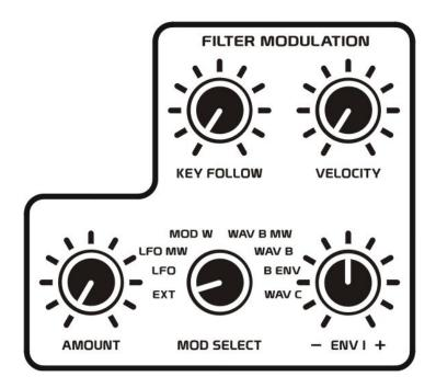
AMOUNT: The amount control sets the amount of modulation that the MOD SELECT source will have on the filter's cutoff frequency. When this control is rotated fully counter-clockwise, no modulation will occur. As you rotate this control clockwise, the amount of modulation will increase.
