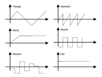
The Flat waveform is a non-oscillating flat LFO, which output is always set to a steady maximum. This is useful as a base for external MIDI control messages.
