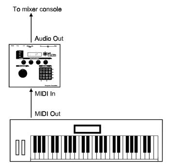
The following setup could be used to connect the SidStation to a computer sequencer:
