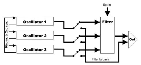
In this manual we speak of an oscillator as a complete set of synthesis components. This means that inside every oscillator we have a tone generator, envelope, pulse width modulation and pitch settings among other things. If the above picture and synthesis terminology seems alien to you, don't be alarmed. Everything will be explained, as we now take an in-depth look at the programming of the SidStation.
