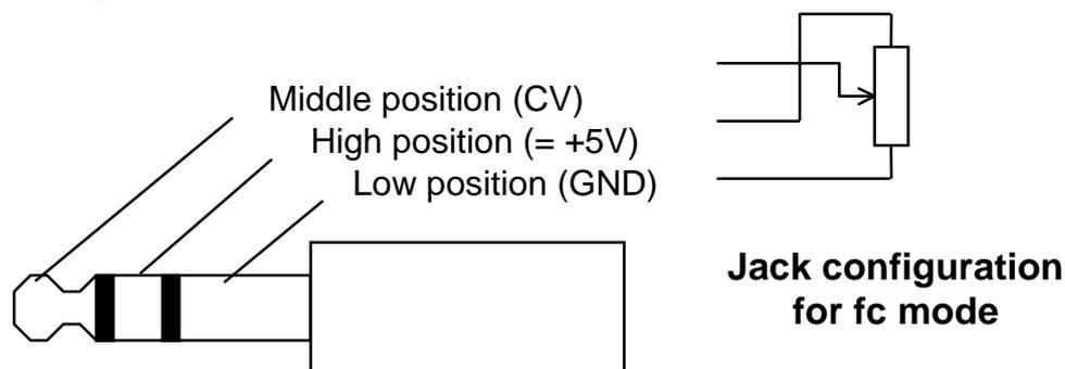
Be careful as to which foot controller you buy, make sure that it is compatible with the **Drehbank**. We recommend the Doepfer FP5/DB foot controller (special version for the **Drehbank**, the FP5 version used with our keyboards is not compatible as the jack connection is different!).
