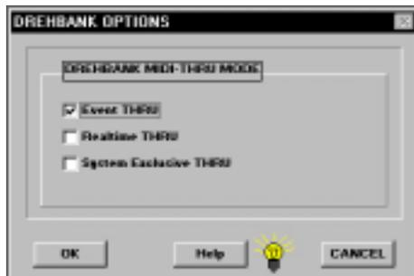
The Midi Thru Mode in the **Drehbank** determines which type of MIDI messages "get-THRU-ed" from the **Drehbank** Midi Inputs to the **Drehbank** Midi Outputs.
