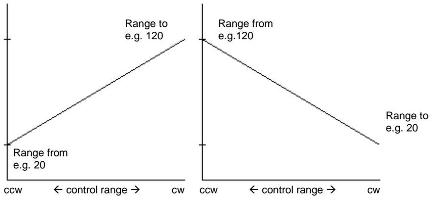
The left picture shows an example with Range from = 20 and Range to = 120. If the knob is turned from left (ccw) to right (cw) the data 20...120 are generated.
