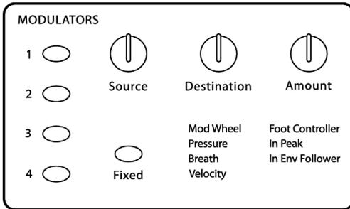
The Modulators section lets you configure the modulation routing and amount for the Poly Evolver's four general-purpose modulation slots as well as for MIDI controllers such as the Mod Wheel, Key Pressure, Velocity, Breath Control, and more.
