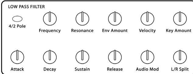
The analog (*real* analog!) lowpass filter is actually two different filters; one for the Left channel and one for the Right channel. This allows true stereo processing of external audio signals run through Evolver. However, for simplicity and consistency the two filters are normally driven together in tandem, so they normally respond the same way.
