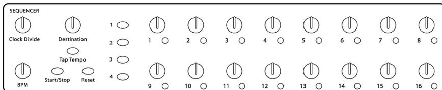
The Poly Evolver features a 4 x 16 “analog-style” step sequencer that can generate four separate sequences of up to 16 steps each. Individual sequences can be routed to any standard modulation destination (see the table on page 41). Using VCA Envelope as a destination, for example, varies the volume of each step; a destination of Filter or Filter Envelope Amount will produce different filter settings per step. Typically, however, at least one sequence is routed to an oscillator to control pitch.
