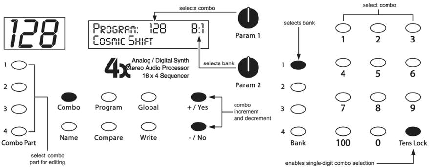
To edit the Combo parameters, first hit the desired COMBO PART Switch. The PARAM 1 knob now selects the parameter, and the PARAM 2 knob changes the value. The + and – switches will increment/decrement the value also. See the Combo Parameters section for a detailed list of all parameters and their functionality.
