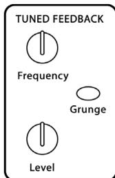
Feedback is implemented via two identical tuned delay lines, one for each channel. See the diagram on page 13 for details on the signal path. Since the delay is tuned, it can be played by modulating the feedback frequency, from the sequencer or other sources.
