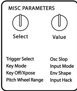
The Misc Parameters section lets you configure a variety of parameters not found elsewhere. The parameter list is printed on the panel as seen above.
