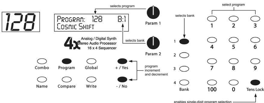
To edit a Program, simply turn any knob while in Program mode. See the Program Parameters section for a detailed list of all parameters and their functionality.
