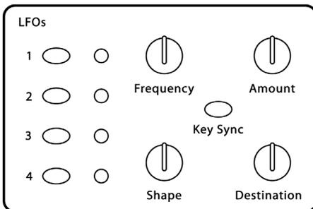
The Poly Evolver has four identical Low Frequency Oscillators (LFOs). To select a specific LFO for editing, press the appropriate switch, 1–4. Turning a knob will then adjust the parameters of the selected LFO. Holding one of the four switches will solo that LFO (the switch will blink) by setting the Amounts of the other three to zero. It does not affect any modulation that is routed to LFO Amounts, though, so at times it may not completely turn off all other Amounts.
