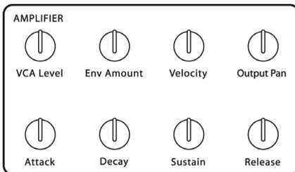
**VCA Level:** *0...100* – Sets a base level for the VCA (Voltage controlled Amplifier). This allows the VCA to be essentially bypassed, which may be necessary for processing external audio signals, or for Programs that drone.
