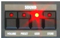
The Preset administration will be handled within the sound section of the Configuration-strip. There are 128 user and 128 factory presets. Actuate the preset button. Use the DOWN/UP button or data wheel to scroll through the presets. A preset
