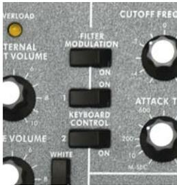
Here you can activate additional Filter-Modulation. The source will be the signal defined within the Modulation-Mix section. This can be Oscillator 3, Noise or a mix of both. Intensity can be adjusted by using the Modulation-Wheel and its additional parameters.
