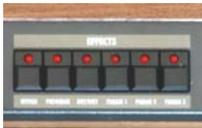
Activate the BYPASS button to bypass any effects. Depending on your adjustments made the signal without effects might be a little bit louder than with effects turned on.
