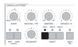
You can definitely see why this waveshape bears the name "sawtooth." Press and hold a key and slowly turn the pot clockwise. You should be able to hear how the tone becomes increasingly more hollow-sounding. You might say this effect thins the sound out, but in any case, the entire tonal spectrum is affected by an equal measure, which is an audio result filters are unable to achieve.
